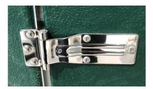
The pre-drilled holes for the hinge bolts are sealed to prevent any possible water ingress to the core material of the door. On painted doors, the door is painted before the hinges are assembled onto a bed of sealant on the door resulting in a corrosion resistant layer. Ensure each hinge bolt is tight to maintain a good seal of the hinge to the door, it is important that every bolt is checked and tightened to ensure all bolts are distributing the load of the door to the frame.
